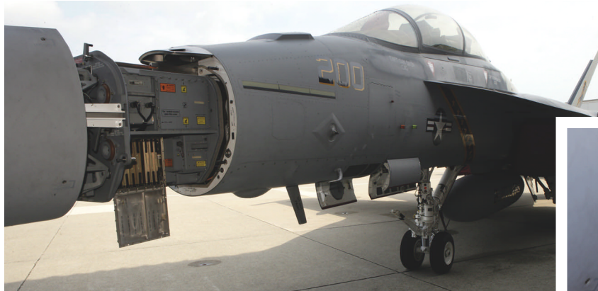
This photograph taken at Naval Air Station Oceana shows the APG-79 AESA radar installed in an F/A-18 Super Hornet. Inset: a Navy maintainer works with the radar. Courtesy of Boeing.
