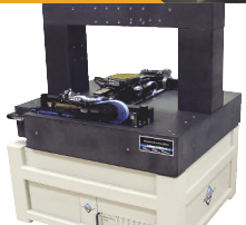
Multi-axis air-bearing with granite bridge and a machine base
